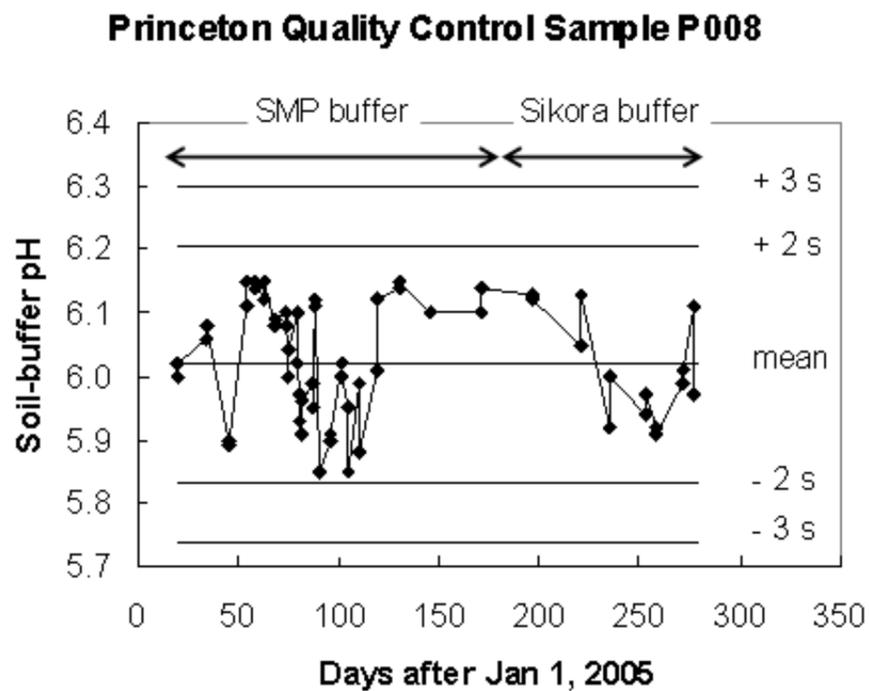
**Figure 2. Quality control charts for soil-buffer pH for samples used in the Lexington and Princeton laboratories. The Sikora buffer has been used since July 1, 2005 (day 182). The mean,  $\pm 2s$ , and  $\pm 3s$  are statistics developed from the SMP buffer data prior to day 182.**
