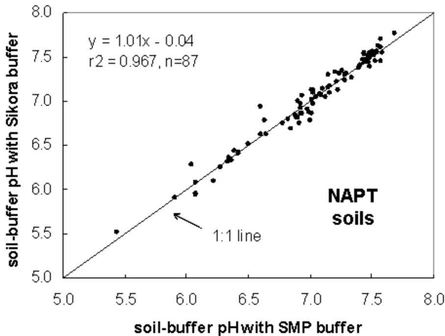
**Figure 1. Comparison between soil-buffer pH with the Sikora buffer and soil-buffer pH with the SMP buffer for 255 Kentucky soils and 87 NAPT soils.**
